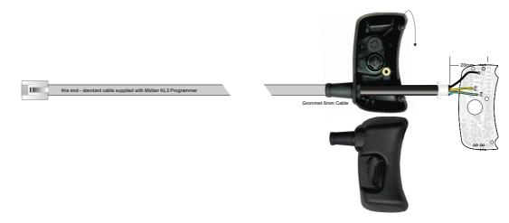
*Note:* This cable uses the standard cable supplied with the KL3 Programmer. Its length is reduced to 900mm by trimming the end with the black, green and yellow wired clips.
